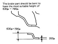
\* The spring is  $200\mu$  in thickness, which you may find helpful when bending the two parts.
