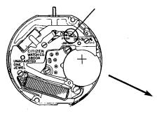
The setting stem should be removed only when it is in its normal position.
